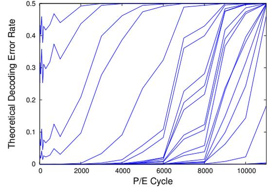
Fig. 4: The theoretical decoding error rates of some subchannels at different PECs. Each curve is for one subchannel.
