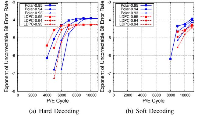
Fig. 2: Comparison between polar codes and LDPC codes.
