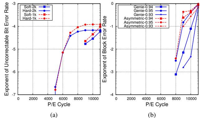
Fig. 3: The performance of polar codes with (a) different block lengths as well as (b) realistic and genie soft sensing.
